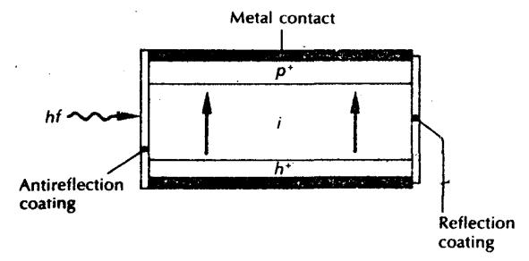
Light is injected parallel to junction plane. This exhibits large absorption width (= $500\mu m$ ) This device is sensitive at wavelength of 1.09 $\mu m$ , where absorption coeff. is relatively small.
