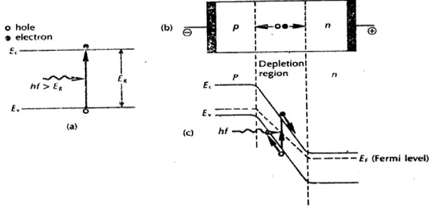
Operation of the p-n photodiode: (a) photogeneration of an electron-hole pair in an intrinsic semiconductor; (b) the structure of the reverse biased p-n junction illustrating carrier drift in the depletion region; (c) the energy band diagram of the reverse biased p-n junction showing photo-generation and the subsequent separation of an electron-hole pair.
