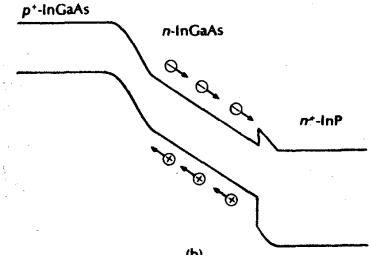
Fabricated as **mesa structure** which reduces parasitic capacitances. Charge trapping at interface causes limitation in response time.
